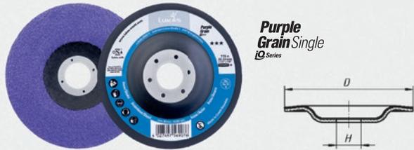
The integrated backing pad made of environmentfriendly recycled fibre guarantees a high degree of stability and durability. The innovative structure allows for uniform wear and tear without overheating, embrittlement or grain shedding. The deep offset zone allows you to work at a flat angle. Thanks to its special tool geometry, the „Purple Grain Single“ can also reach inaccessible areas, thus offering more possible applications than a conventional tool.
